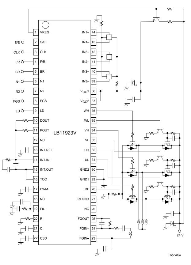
Sample Application Circuit 1 (P-channel + n-channel, Hall-effect sensor application)
